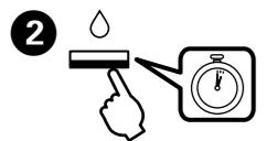
Run the print head cleaning. Hold down  $\odot$  for **3 seconds** until  $\odot$  starts flashing.
